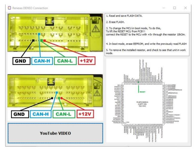
After writing flash, the resistor must be removed.
