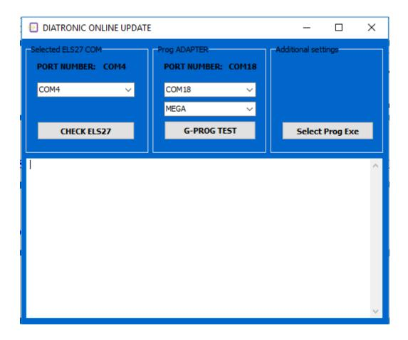
In the settings menu, select the COM PORT on our adapter, and close the window, when the window is closed, the program will create a ini file with the settings and remember the port number.
