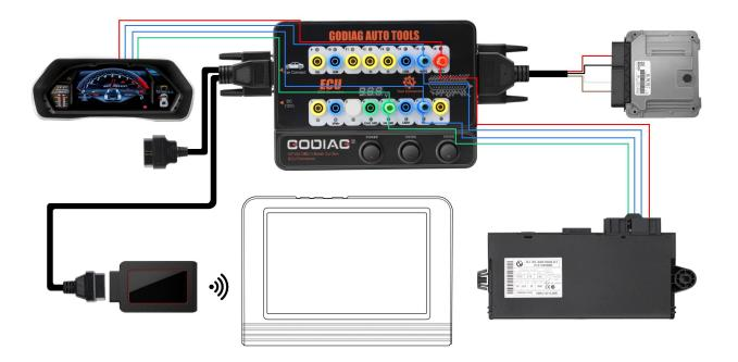
6. When to use the extension cables: The space of the diagnostic interface location is too narrow to connect to the diagnostic tool, or the user find that the diagnostic cable is not long enough during maintenance. It can be extended by 1.2 meters.
