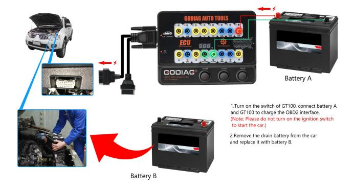
1). Prepare battery A to supply power by connecting to No. 16 / 4 / 5 holes of Godiag GT100 & to the OBD2 diagnostic interface of the car.
