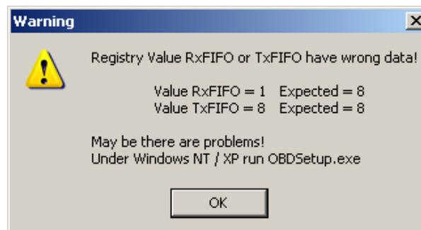
**Reason:** The value of the variable DWORD (here RxFIFO) can not be set by OBDSSetup.exe.
