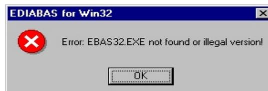
This error occurs if the path variable is set with the path C:\EDIABAS\BIN in the system and user variables (Start à My Computer à Control Panel à System à Advanced and then in the "Environment" tab).
