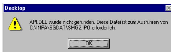
Reason: The path C:\EDIABAS\BIN has not been set in the 'Path' system variable.
