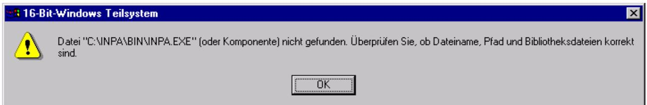
Reason 1: The path C:\EDIABAS\BIN has not been set in the 'Path' system variable.
