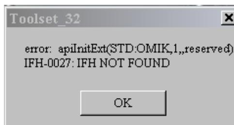
Reason 4: The old OMITEC driver wasn't uninstalled correctly.
