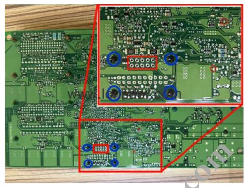
Type A: open the lid, pay attention to the black columns in the blue circle on the back of the circuit board, those are four positioning points, stably match them respectively with the white columns on RN-01 board.
