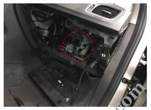
Volvo's CEM is basically located behind the storage box which is in front of the co-pilot seat
