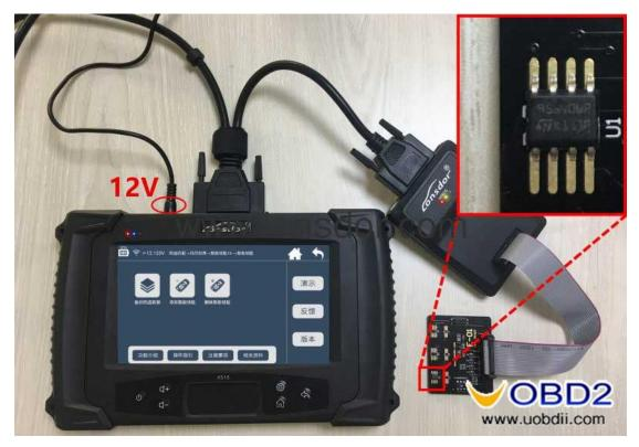
**Note:** If you can not read data with the KPROG adapter, you can use a programmer to read and copy the data into the K518ISE specified folder, the path: K518 -> file -> feature\_553
