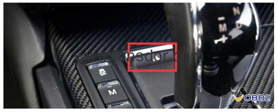
For the new Maserati models, in the bottom of the pole position has a "knob" as shown below, cars without this knob belong to the old system before 2016.
