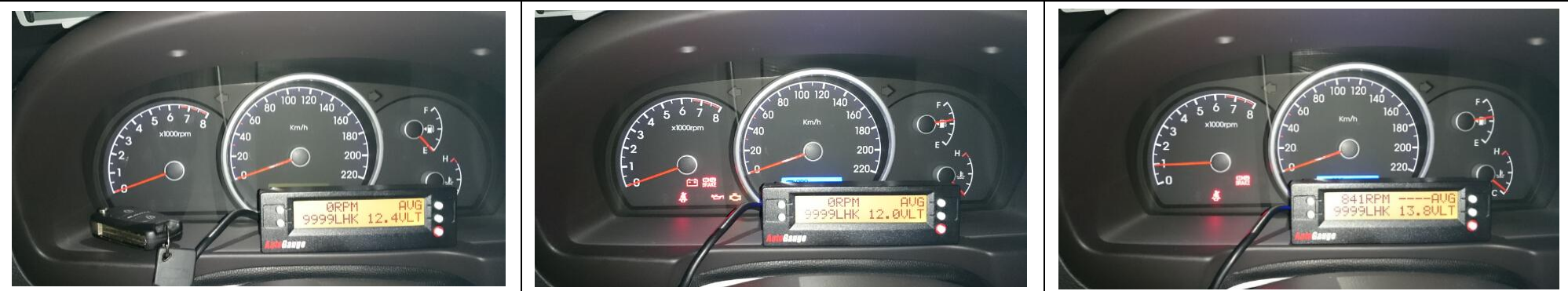
Auto power off and car key no insert, reading voltage as 12.4V
