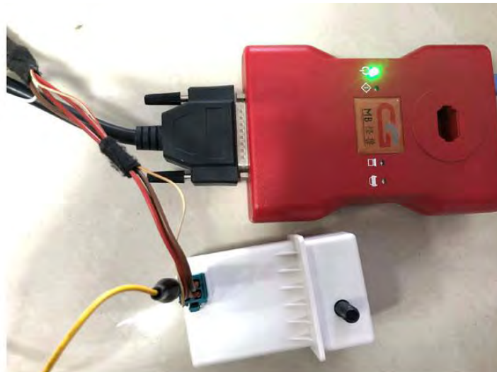
Put on the simulator and clip the K-line
