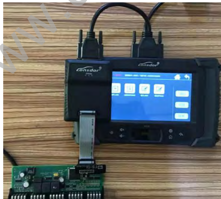
Connection between K518ISE host, adapter and FS-01 board:
