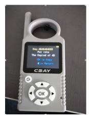
6. Put 4D clone able chip into signal coil, press "OK" button.
