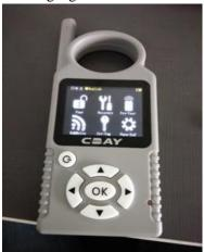
2. Put the key into signal coil area and use arrow button to select "COPY", then wait, it is copying.
