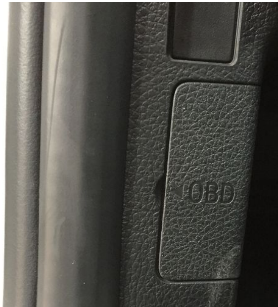
Picture1. OBD diagnosis socket of BMW 1 series
