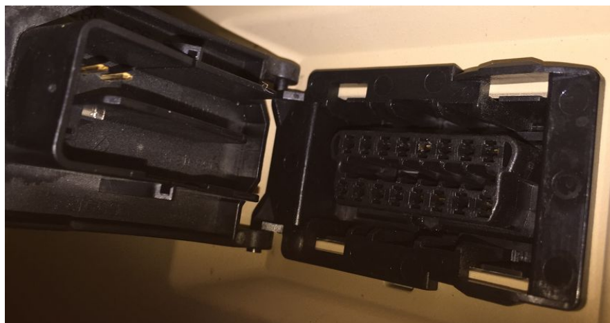
Picture4. OBD diagnosis socket of BMW 7 series
