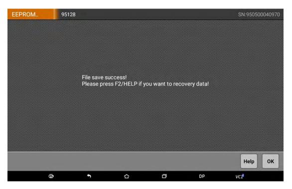
Notice: The original EEPROM data backup completed and saved with the name "FEM00000". Disassemble 95128/95256 chip from adapter board and weld back to FEM/BDC module.
