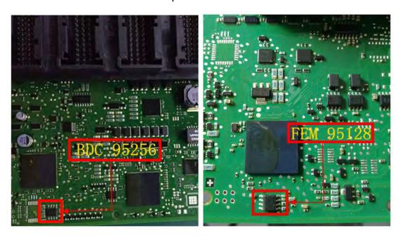
Weld the 95128/95256 chip to the 95XXX position on the adapter board or insert to the chip holder with the chip clip, (pay attention to the direction of the chip) as following:
