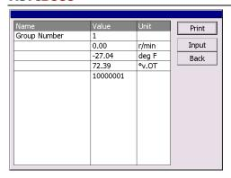
Note: Under basic setting mode, you can perform solenoid and engine control unit adaptation without starting the engine, or finish  $\lambda$  control process self-adaptation when engine starts. Also you can check faults or ignition timing by connecting or disconnecting  $\lambda$  control.
