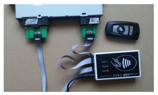
$\square$ . After make new key, put it on the sensing area of test platform device, within 10 seconds the LED3 indicator will be on, the key is identified.
