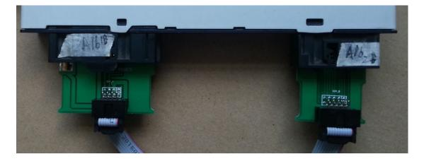
—. When CAS4 box is connected to the test platform device, the device system will automatically test whether CAS4 box is working or not. If LED2 indicator won't flash, it indicates the CAS4 box is not working. The solution is to check whether 5M48H is welded ok after pinout.
